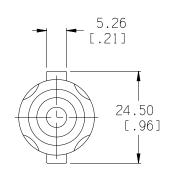
SPECIFORM: ON 6, FLAMMABILITY RATING UL94V-0 UL FILE NO. E154352
