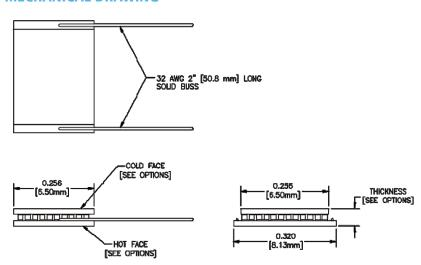
Solder Construction: 138°C, Bismuth Tin Tlam Substrates
