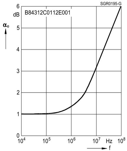
**Insertion loss  $\alpha_e$  in stopband (typical)**
