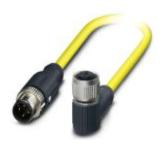
Sensor/Actuator cable, 4-position, PVC, Yellow RAL 1021, shielded, Plug straight M12-SPEEDCON, A-coded, on Socket angled M12-SPEEDCON, A-coded, Cable length: 0.5 m
