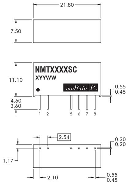
All dimensions in mm  $\pm 0.25$ mm. All pins on a 2.54 pitch and within  $\pm 0.25$  of true position. Weight: 3.85g
