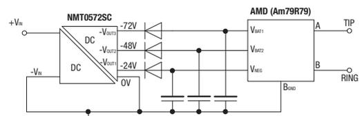
Figure 2. Supply for Ringing SLIC Device
