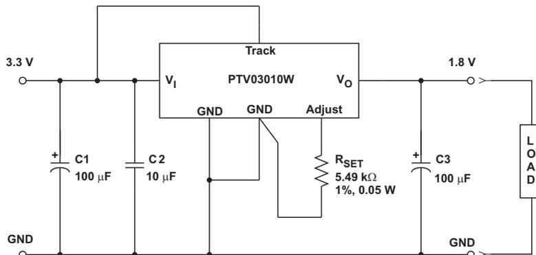
**Figure 7. Power-Up Application Circuit**
