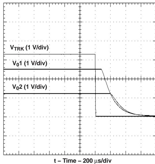
Figure 13. Simultaneous Power Down With Auto-Track Control
