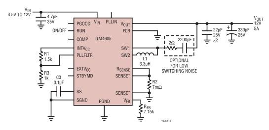
Figure 15. Boost Mode Operation with 4.5V to 12V Input
