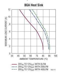
Figure 12. 20V<sub>IN</sub> to 12V<sub>OUT</sub> with Heat Sink
