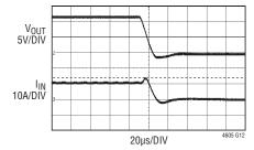
OUTPUT CAPS:  $22\mu F \times 4$  CERAMIC CAPS AND  $180\mu F \times 2$  ELECTROLYTIC CAPS  $15m\Omega \times 2$  SENSING RESISTORS
