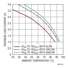
Figure 9. 5V<sub>IN</sub> to 16V<sub>OUT</sub> without Heat Sink
