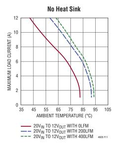
Figure 11. 20V<sub>IN</sub> to 12V<sub>OUT</sub> without Heat Sink
