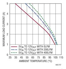
Figure 7. 5V<sub>IN</sub> to 12V<sub>OUT</sub> without Heat Sink
