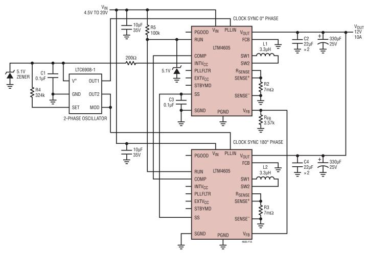
Figure 18. Two-Phase Parallel, 12V at 10A Design
