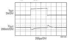
LOAD STEP: 0A TO 3A AT CCM OUTPUT CAPS:  $22\mu F \times 4$  CERAMIC CAPS AND  $180\mu F \times 2$  ELECTROLYTIC CAPS  $15m\Omega \times 2$  SENSING RESISTORS
