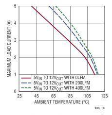
Figure 8. 5V<sub>IN</sub> to 12V<sub>OUT</sub> with Heat Sink
