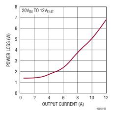
Figure 6. 20V<sub>IN</sub> Power Loss
