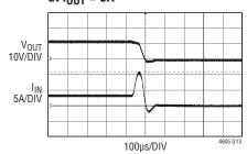
OUTPUT CAPS:  $22\mu F \times 4$  CERAMIC CAPS AND  $180\mu F \times 2$  ELECTROLYTIC CAPS  $15m\Omega \times 2$  SENSING RESISTORS
