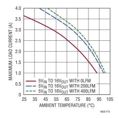
Figure 10. 5V<sub>IN</sub> to 16V<sub>OUT</sub> with Heat Sink
