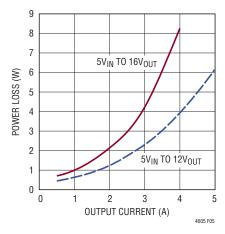
Figure 5. 5V<sub>IN</sub> Power Loss
