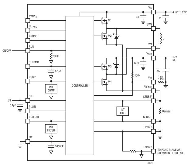
Figure 1. Simplified LTM4605 Block Diagram
