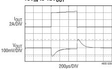
LOAD STEP: 0A TO 4A AT CCM OUTPUT CAPS:  $22\mu F \times 4$  CERAMIC CAPS AND  $180\mu F \times 2$  ELECTROLYTIC CAPS  $15m\Omega \times 2$  SENSING RESISTORS
