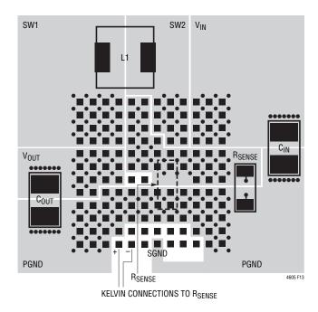
Figure 13. Recommended PCB Layout
