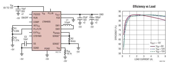
Figure 19. Buck Mode Operation with Positive Input to Negative -5V Output Converter
