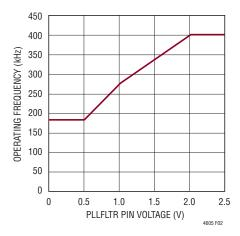
Figure 2. Frequency vs PLLFLTR Pin Voltage
