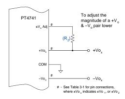
Table 3-1; Adjust Resistor Pin Connections
