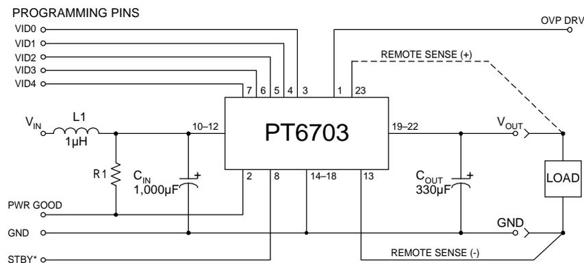
C<sub>in</sub>/C<sub>out</sub>: Required electrolytic capacitors –see footnotes.
