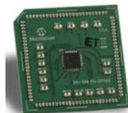
This PIM comes with a 28-pin dsPIC33FJ16GP102 QFN device. Use with the Explorer 16 Development Board (DM240001 or DM240002).
