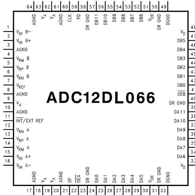
Figure 1. 64-Lead TQFP Package
