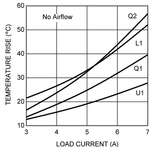
Figure 4. Temperature Rise at 24V<sub>IN</sub> with 5.6 µH Pulse Inductor
