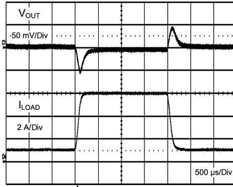
Figure 12. Transient Response at 24V<sub>IN</sub>
