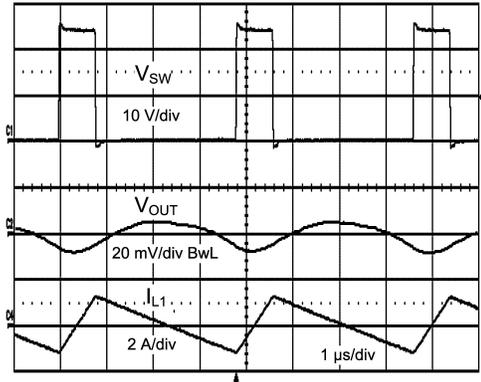
Figure 10. Full Synchronous Operation at 24V<sub>IN</sub> with JMP1 Removed
