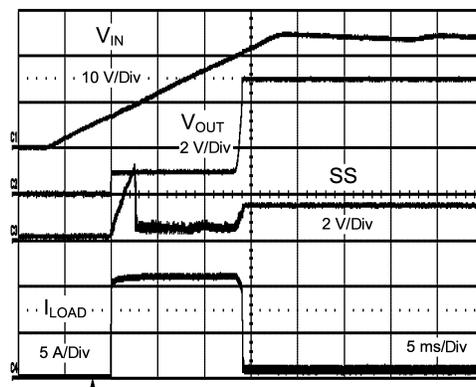
Figure 9. Start-up into Active Load at 24V<sub>IN</sub>
