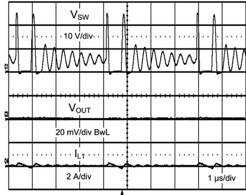
Figure 11. Discontinuous Operation using Diode Emulation Mode at 24V<sub>IN</sub> with JMP1 Installed
