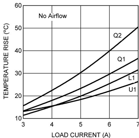
Figure 3. Temperature Rise at 24V<sub>IN</sub> with 6 µH Cooper Inductor
