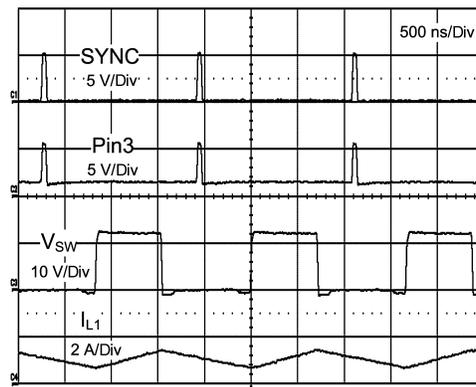
Figure 8. Synchronization at 12V<sub>IN</sub>
