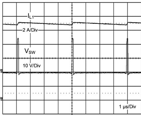
Figure 5. Short Circuit at  $24V_{IN}$  Room Temperature
