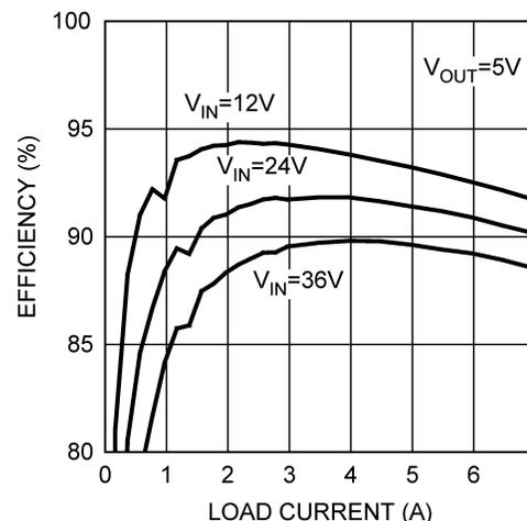
**Figure 2. Efficiency with 5.6 µH Pulse Inductor**
