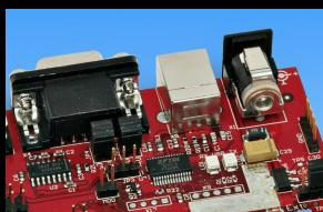
■ The MB96F338U microcontroller offers USB-Host/-Function that is supported by SK-16FX-144PMC-USB
