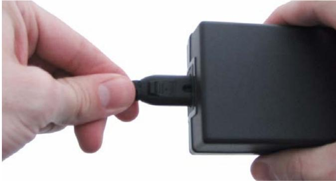
3. Plug the power adapter into an electrical outlet and the 5V line output connector into the power-in connector on the baseboard.
