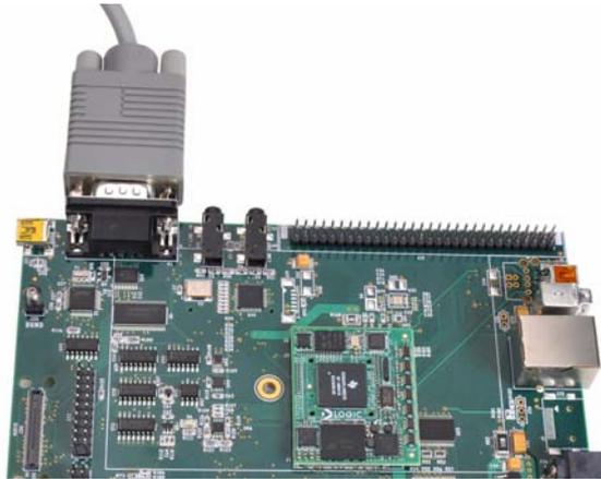
2. Connect the regulated 5V power supply to the appropriate power adapter for the region in which you are using the eXperimenter Kit.
