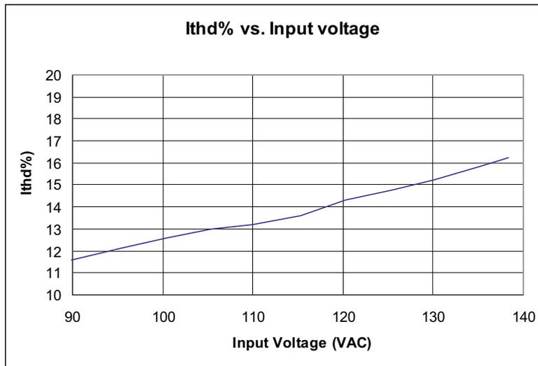
Figure 7. I<sub>thd</sub>% vs Input Voltage
