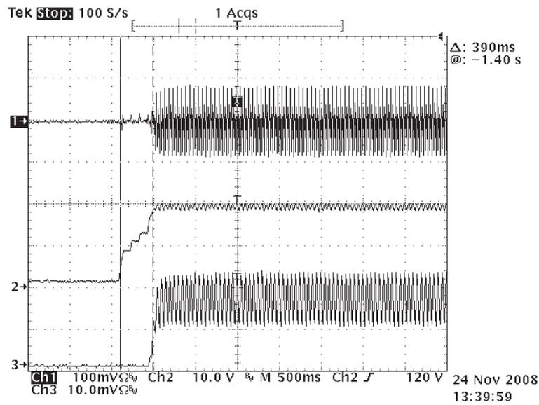
**Figure 13. Enable Turn-On Delay**
