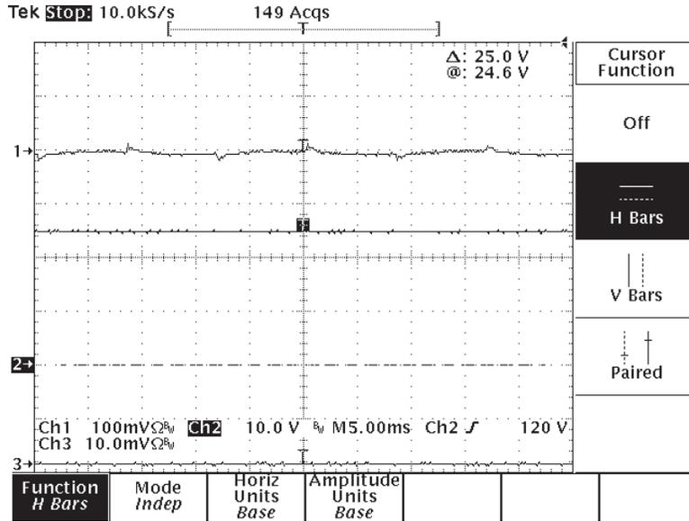
**Figure 15. LED Open Circuit Waveforms**
