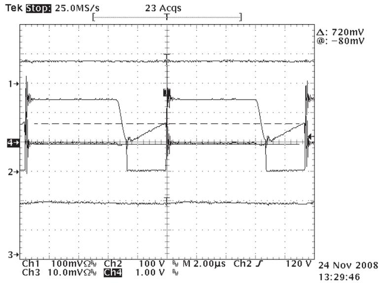
**Figure 11. Current Sense Waveform**
