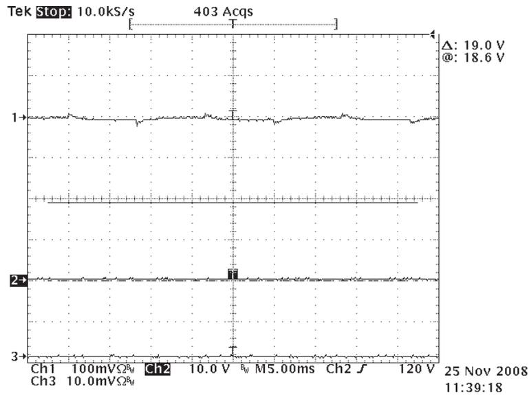
**Figure 16. LED Short Circuit Waveforms**
