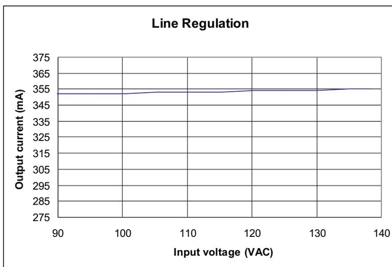
Figure 5. Current Variation with Respect to Input Voltage
