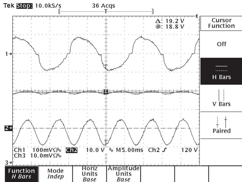
**Figure 14. Pre-Open and Short Circuit Waveforms**
