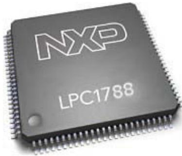
The NXP LPC1788 Cortex M-3 based microcontroller runs the open source  $\mu$ EZ<sup>®</sup> + FreeRTOS software platform. The LPC1788 has 512KB of internal Flash memory, 96KB of internal SRAM, a 10/100 Ethernet Media Access Controller (MAC), a USB full speed device/host/OTG controller, four UARTs, two CAN channels and a collection of serial communications interfaces. The  $\mu$ EZ GUI board also includes 8MB of external SDRAM and 8MB of external NOR Flash.
