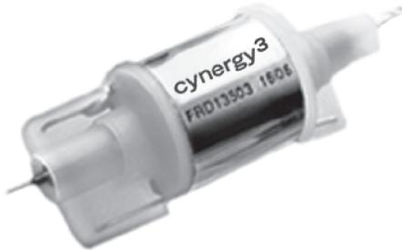
A complete RF screen around the coil assembly for a low loss transmission path, results in better carry current at elevated temperatures for this open frame series. An anti-corona sleeve is fitted around the reed switch for improved RF voltage isolation. This type is widely used in HF Antenna Tuning Unit (ATU) applications.
