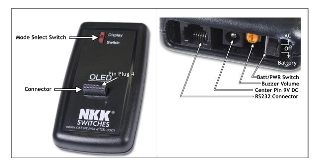
The **Mode Select Switch** has two settings; "Switch" is for the OLED (64x48) switches and "Display" is for the OLED (52x36) displays.
