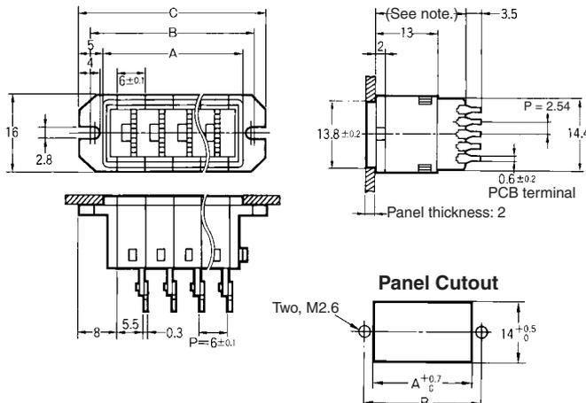
Note: If the output code is 06, the dimension is 19; if the output code is 07, the dimension is 31.
