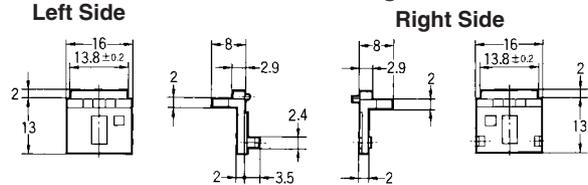
**Note:** The A7MD cannot be mounted by a screw panel or snap-in panel. Fasten the PC board after mounting the A7MD to the PC board.
