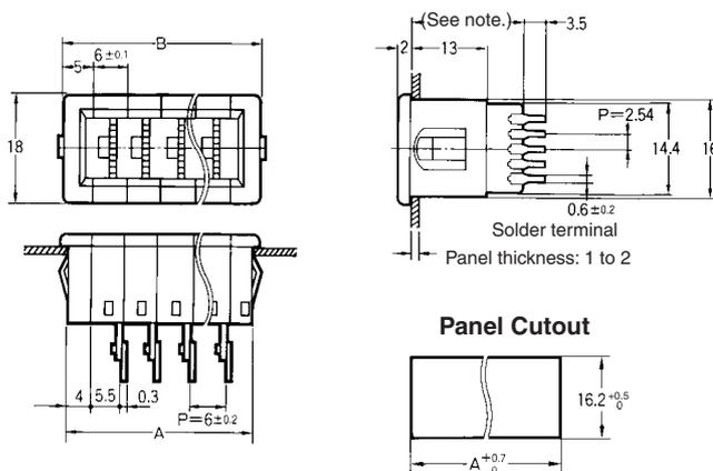
**Note:** If the output code is 06, the dimension is 19; if the output code is 07, the dimension is 31.
