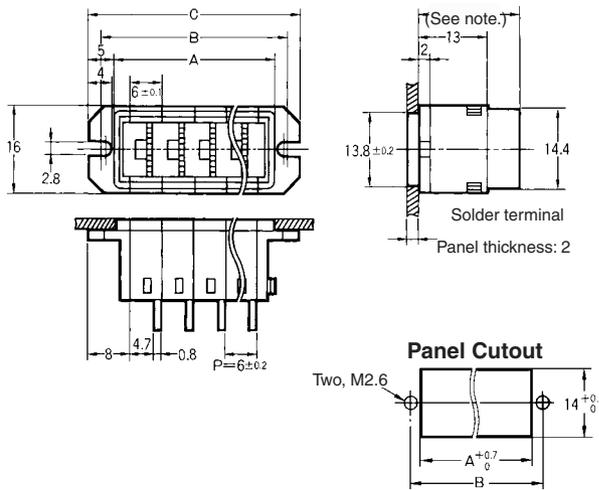
Note: If the output code is 06, the dimension is 19; if the output code is 07, the dimension is 31.
