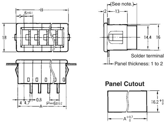
**Note:** If the output code is 06, the dimension is 19; if the output code is 07, the dimension is 31.
