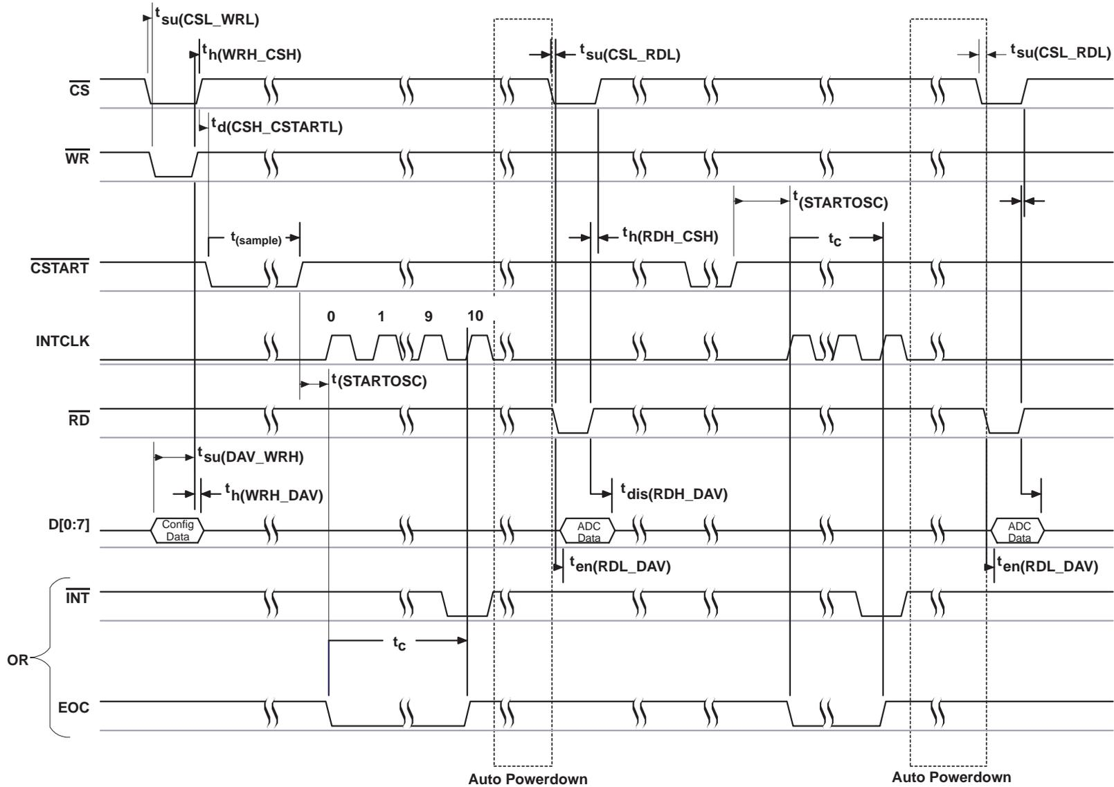
**Figure 5. Input Conversion – Hardware  $\overline{CSTART}$ , Internal Clock**
