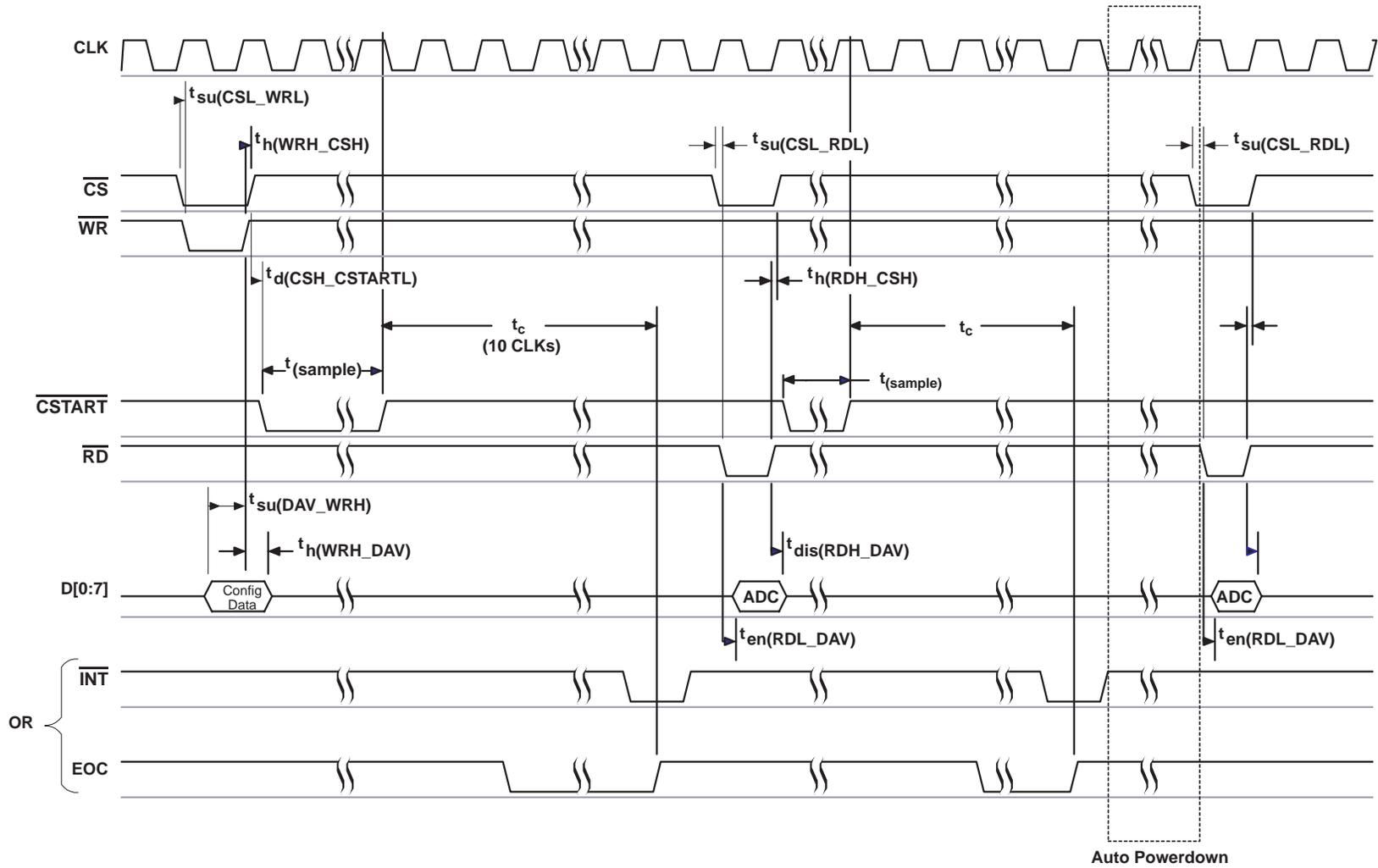
Figure 4. Input Conversion – Hardware  $\overline{CSTART}$ , External Clock
