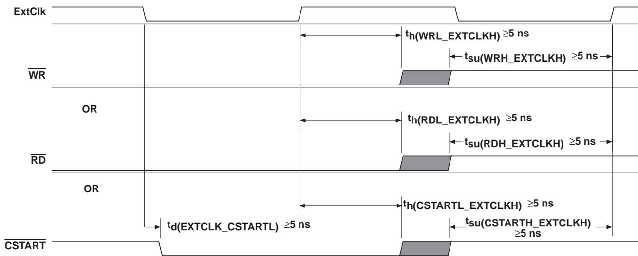
NOTE:  $t_{su}$  = setup time,  $t_h$  = hold time
