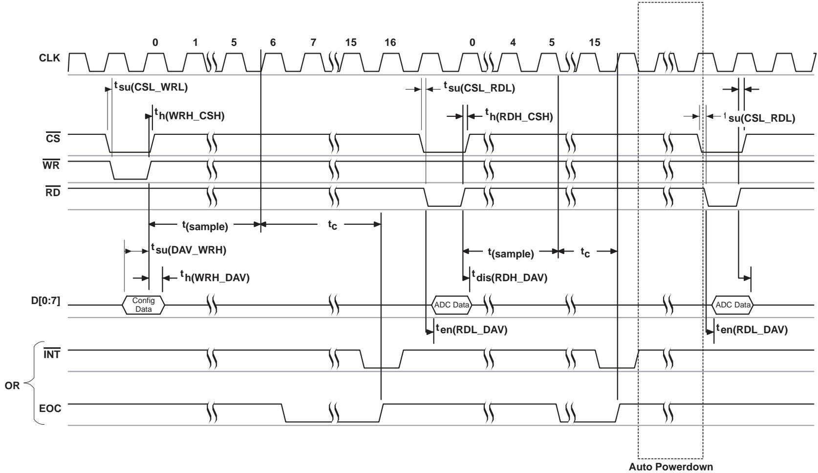
Figure 6. Input Conversion – Software Start, External Clock
