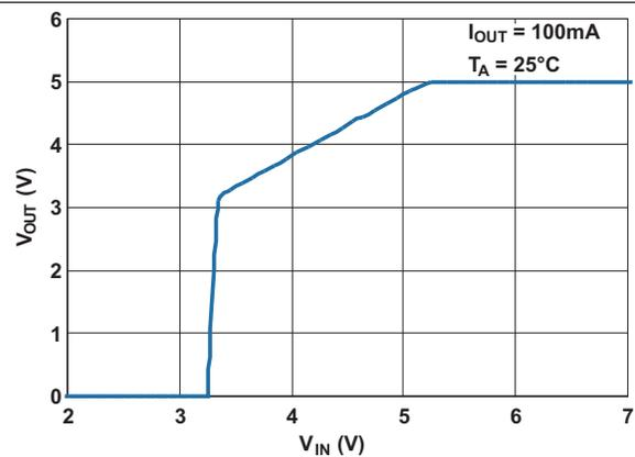
**Figure 8. Output Voltage vs Input Voltage**
