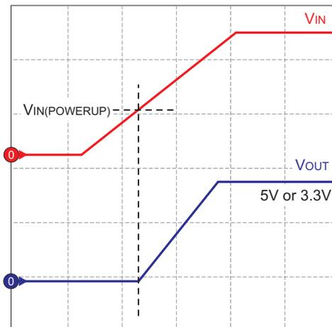
Figure 15. Power-Up Operation
