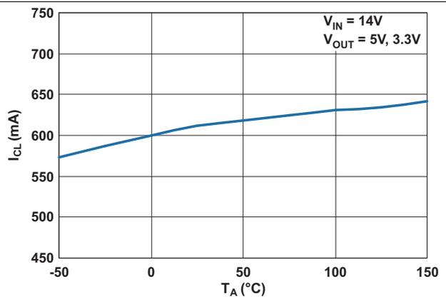
**Figure 10. Output Current Limit vs Ambient Air Temperature**
