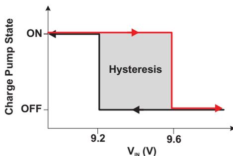
Figure 17. Charge Pump Operation at Heavy Loads
