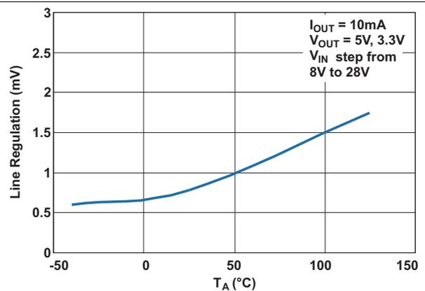
**Figure 12. Line Regulation vs Ambient Air Temperature**
