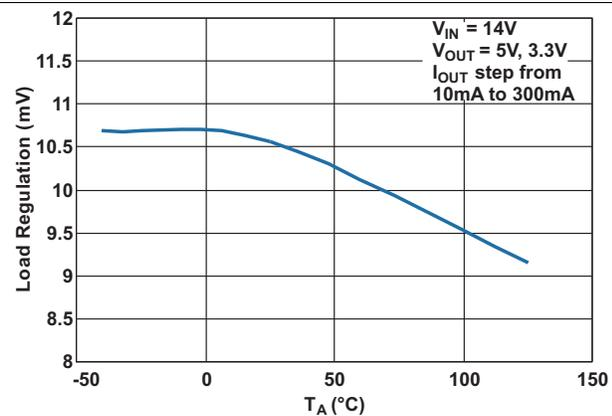
**Figure 11. Load Regulation vs Ambient Air Temperature**
