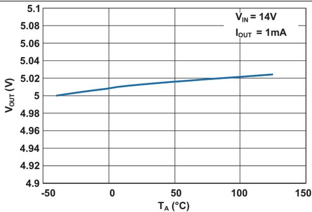
**Figure 7. Output Voltage vs Ambient Air Temperature**
