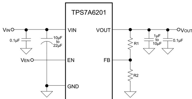
Figure 20. Typical Application Schematic for TPS7A6201-Q1
