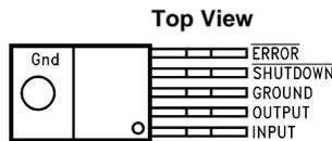
**Figure 1. Bent, Staggered Leads
