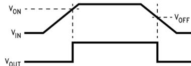
**Figure 33. Snap-On/Snap-Off Input and Output Voltage Diagram**
