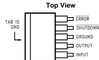
**Figure 2. Plastic Surface Mount Package
