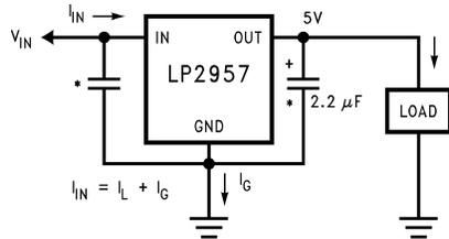
$$P_{TOTAL} = (V_{IN} - 5)V_L + (V_{IN})I_G$$
