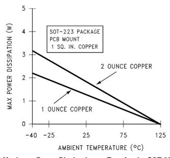
Figure 20. Maximum Power Dissipation vs T<sub>AMB</sub> for the SOT-223 Package
