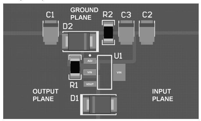
Figure 18. Layout Example (SOT-223)
