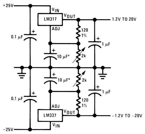
Full output current not available at high input-output voltages \*The 10 µF capacitors are optional to improve ripple rejection
