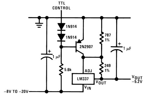
Minimum output  $\simeq -1.3$  V when control input is low
