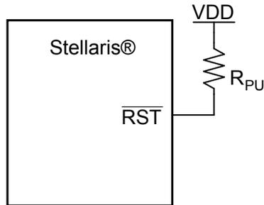
$R_{\text{PU}} = 0$  to 100 k $\Omega$
