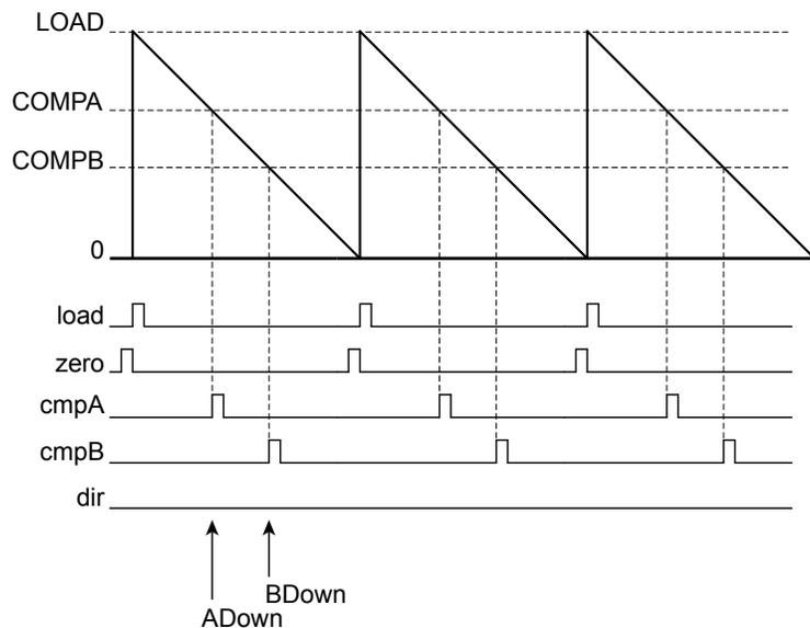
**Figure 20-4. PWM Count-Up/Down Mode**
