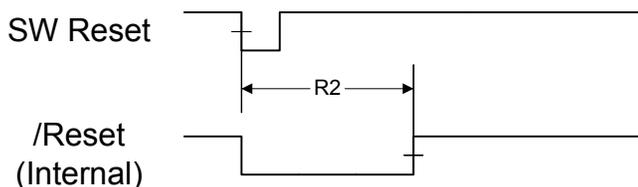
**Figure 25-9. Watchdog Reset Timing**
