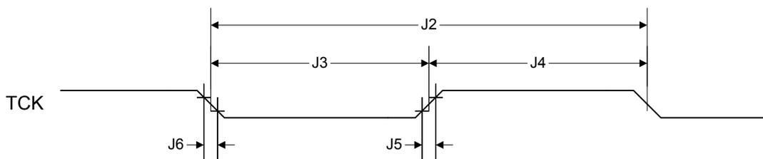
Figure 25-3. JTAG Test Access Port (TAP) Timing
