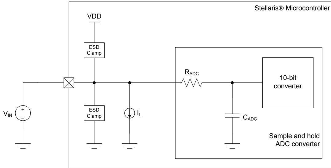
The ADC operates from both the 3.3-V analog and 1.2-V digital power supplies. The ADC clock can be configured to reduce power consumption when ADC conversions are not required (see “System Control” on page 202). The analog inputs are connected to the ADC through specially balanced input paths to minimize the distortion and cross-talk on the inputs. Detailed information on the ADC power supplies and analog inputs can be found in “Analog-to-Digital Converter (ADC)” on page 1110.
