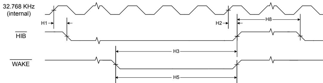
**Figure 25-12. Hibernation Module Timing with Internal Oscillator Stopped in Hibernation**
