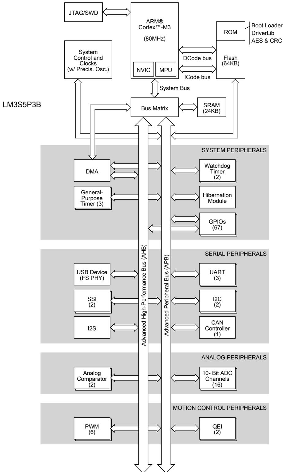
For applications requiring extreme conservation of power, the LM3S5P3B microcontroller features a battery-backed Hibernation module to efficiently power down the LM3S5P3B to a low-power state during extended periods of inactivity. With a power-up/power-down sequencer, a continuous time counter (RTC), a pair of match registers, an APB interface to the system bus, and dedicated battery-backed memory, the Hibernation module positions the LM3S5P3B microcontroller perfectly for battery applications.
