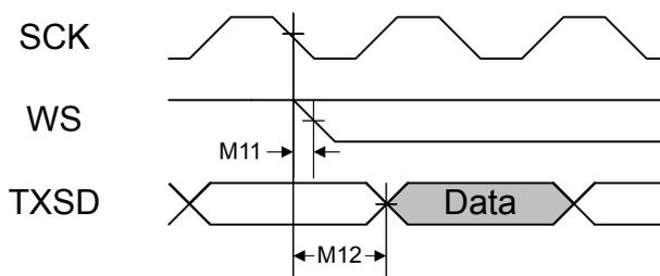
Figure 25-19. I<sup>2</sup>S Master Mode Receive Timing
