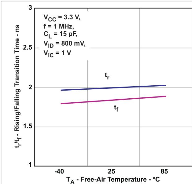
Figure 5-5. Receiver (Type-2) Transition Time vs Free-Air Temperature
