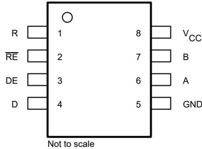
**Figure 4-1. D Package, SOIC 8 Pins
