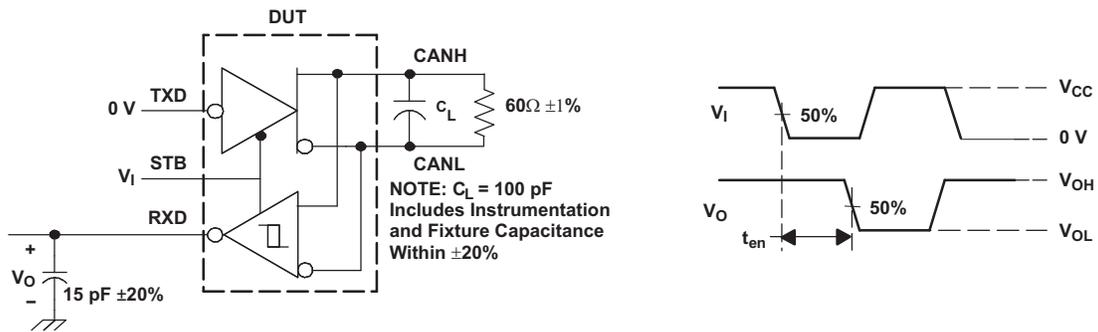
Figure 8.  $t_{en}$  Test Circuit and Voltage Waveforms
