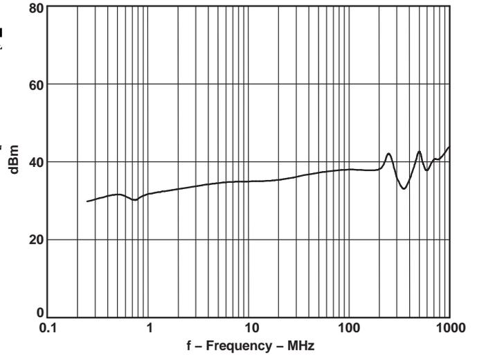
Figure 24. Direct Power Injection (DPI) Response vs Frequency
