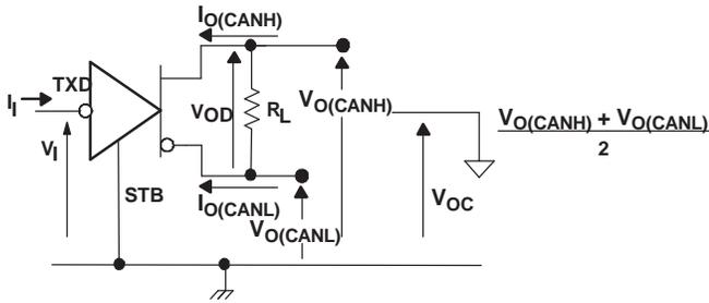
Figure 2. Driver Voltage, Current, and Test Definition
