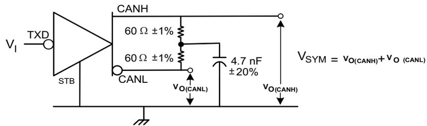
Figure 14. Driver Output Symmetry Test Circuit
