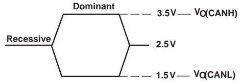
Figure 3. Bus Logic State Voltage Definitions
