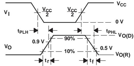
Figure 5. Driver Test Circuit and Voltage Waveforms
