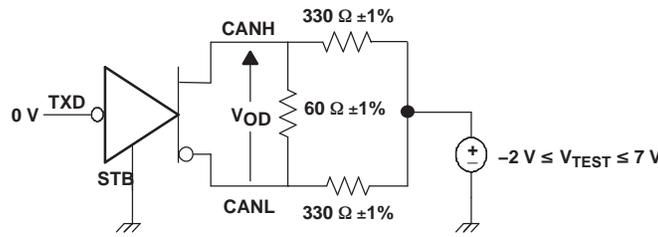
Figure 4. Driver V<sub>OD</sub> Test Circuit
