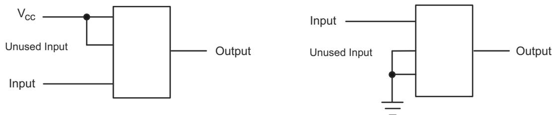
**Figure 11-1. Layout Diagram**
