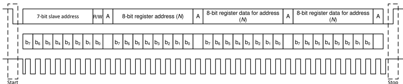
**Figure 7-4. Typical I<sup>2</sup>C Sequence**
