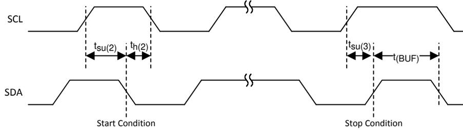
**Figure 6-2. Timing for Start and Stop Conditions**
