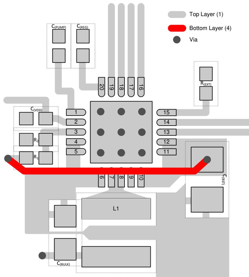
**Figure 10-1. Layout Example with a 4-Layer Board**
