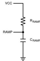
**Figure 8-3. Additional Slope Compensation for  $V_{OUT} > 5\text{ V}$**
