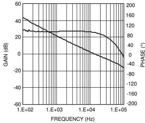
**Figure 8-6. Overall Loop Gain and Phase**
