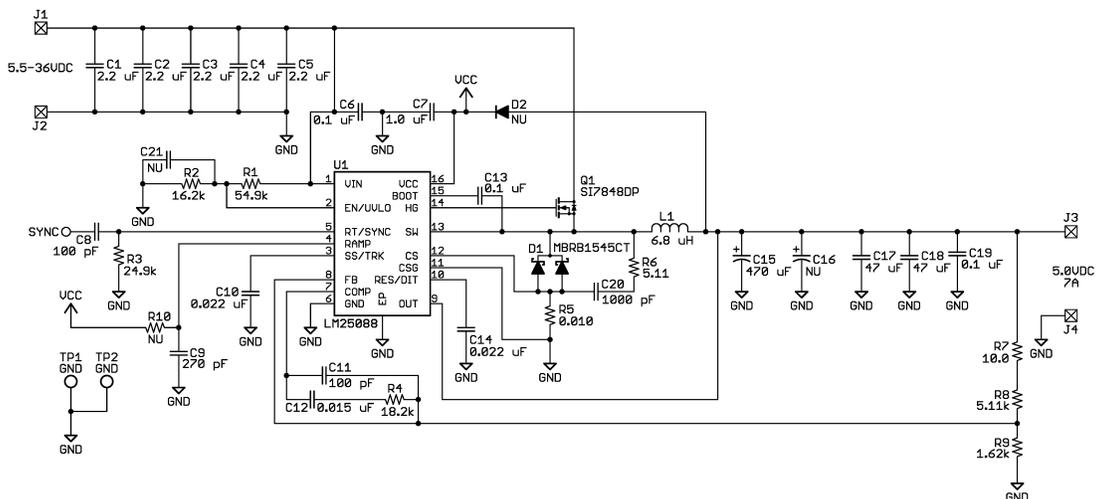
**Figure 9-2. LM25088-2 Application Schematic**
