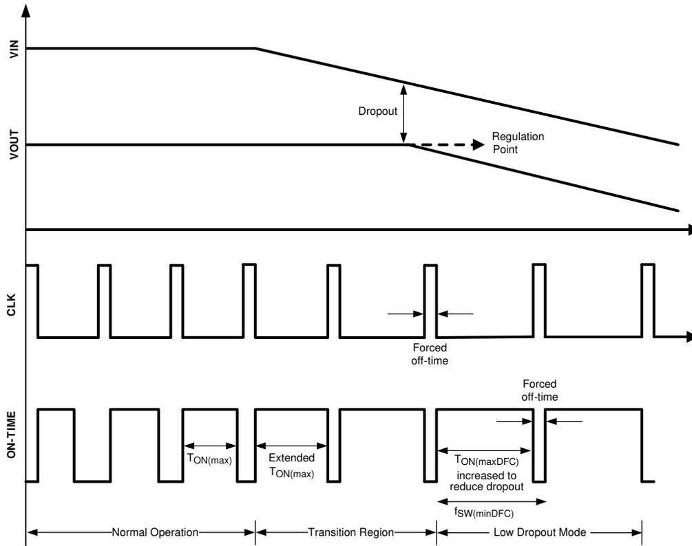
Figure 7-4. Dropout Voltage Reduction using Dynamic Frequency Control
