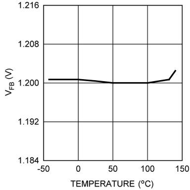
**Figure 6-7. V<sub>FB</sub> vs Temperature**
