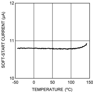
**Figure 6-9. Soft Start vs Temperature**
